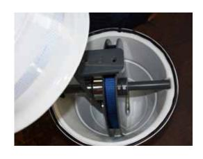
20: Carefully place the upper housing onto the lower housing.
